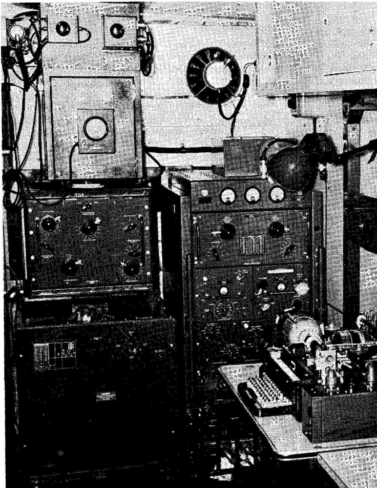
The Royal Signals A.R.S. was recently presented by Marconi's with valuable equipment for amateur-band operation, for use at Catterick Camp, the Hq. of the RSARS. The Tx is a Marconi HS27, giving 350 watts p.e.p., suitable for CW/AM/SSB/RTTY, and the receiver an HR28 double superhet covering 2-30 mc. The presentation was made by Mr. A. W. Laws (manager of the Radio Communications Division of the Marconi Co.) to Brig. A. J. Woodrow, MBE, who commands the Training Brigade, Royal Signals.
