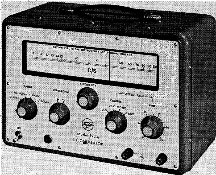
The new Taylor Model 192A LF oscillator has been designed as a general-purpose laboratory signal generator. The range is 10 cycles to 100 kc in four switched bands, the required wave shape being selected by the waveform switch. Maximum sine-wave output voltage is 25v. RMS, with an output impedance of 68 ohms at 25 mV. The instrument is intended as a low power source for checking the frequency and transient characteristics of audio amplifiers and transformers, speakers and similar apparatus. The circuitry involves a Wien bridge with a Schmitt trigger to form the output wave shape.
